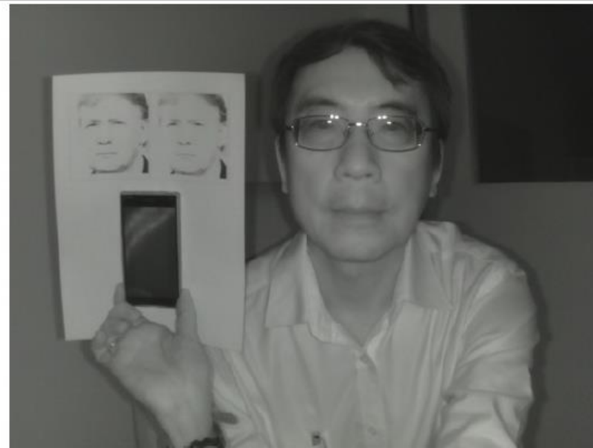
Standard PiCamera with IR-pass filter, and 2x IR LED shining at subject
