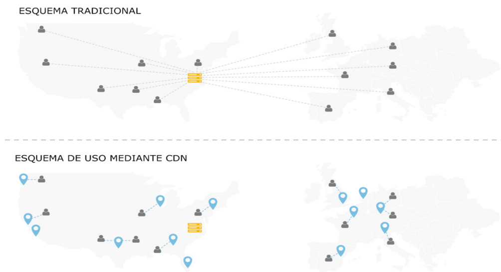
Figure 1 - Diagram of how a CDN network works.
