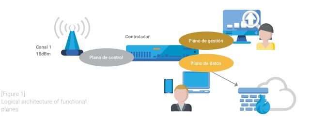
To secure a Wi-Fi network, it is important to know where each of the logical planes is located and how the different elements that form part of the service communicate. Each product and manufacturer's solution has its own architecture definition and it is the administrator's task to know its own characteristics in order to configure it correctly.
