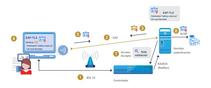
The resulting role may contain settings such as VLAN, firewall filters to apply, bandwidth control, or any other parameters that the network infrastructure allows to be applied. If the server determines that it does not have enough data to decide on the health of the device, it may apply a "validation role" to provide the minimum services necessary to receive a device health status report **(step 7)**.
