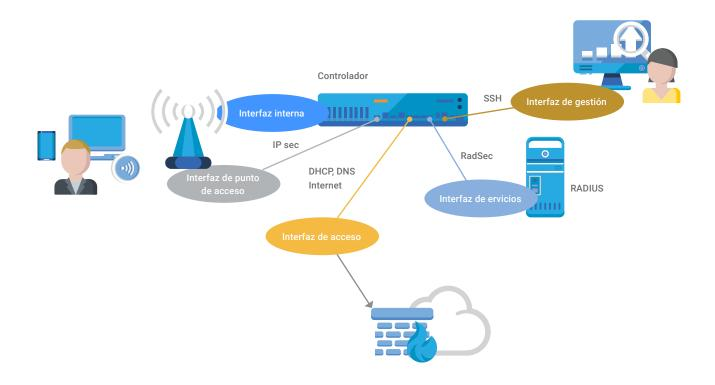
The controller also takes on other control plane tasks such as the orchestration of channel and power allocation. Depending on the vendor solution, certain control plane tasks may be delegated to a server or cloud service outside the controller.
