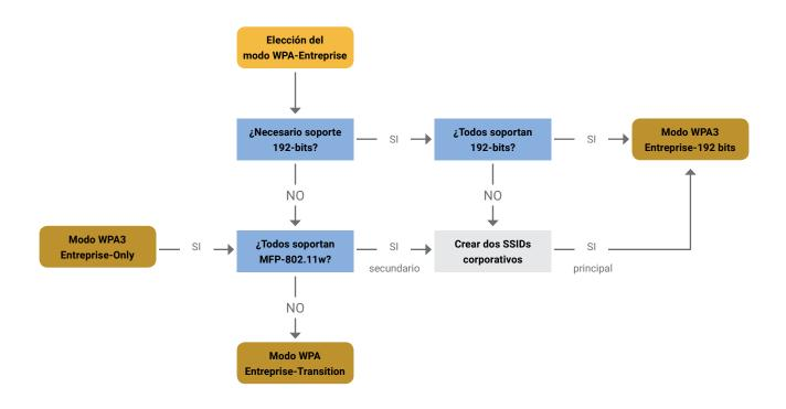
For SSIDs where 192-bit mode is not configured, it is recommended to at least optionally enable all features that are a requirement for 192-bit mode: use of the robust cipher suites, AES-256-GCM encryption and MFP-802.11w.
