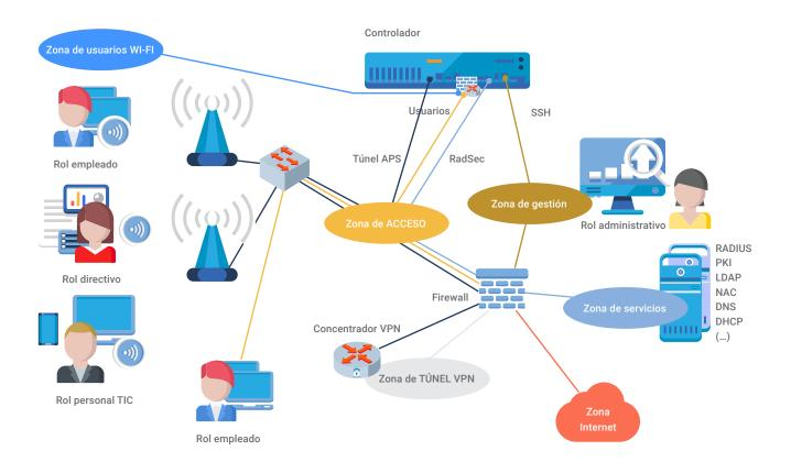
If it is decided that the controller will act as a level 3 equipment (performing routing tasks) two zones can be defined in the controller for the users: Wi-Fi user network zone and corporate access network zone.
