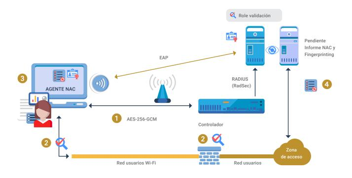
For better analysis and profiling, it is recommended to use a programme, agent or system (NAC agent) installed on the computer of the user who is going to access the network to verify that the terminal to be accessed has minimum security requirements **(step 3)**.
