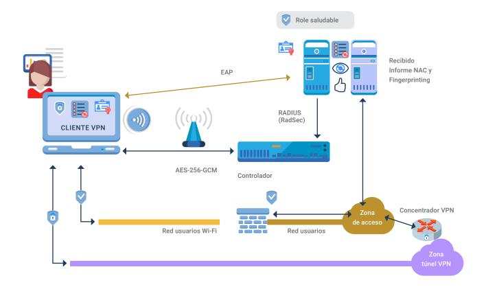
Depending on the solution implemented and its integration with the Wi-Fi solution, the process of association, authentication, status verification and VPN tunnel establishment may be performed with a single agent or application.
