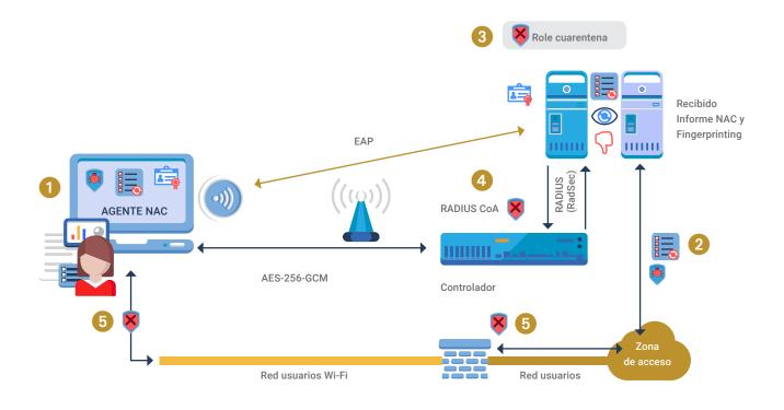
If, on the other hand, the report indicates that it does not comply with the security requirements, it will switch to **"quarantine role"**, restricting access to the minimum services required to solve the problems detected **(Figure 10)**.
