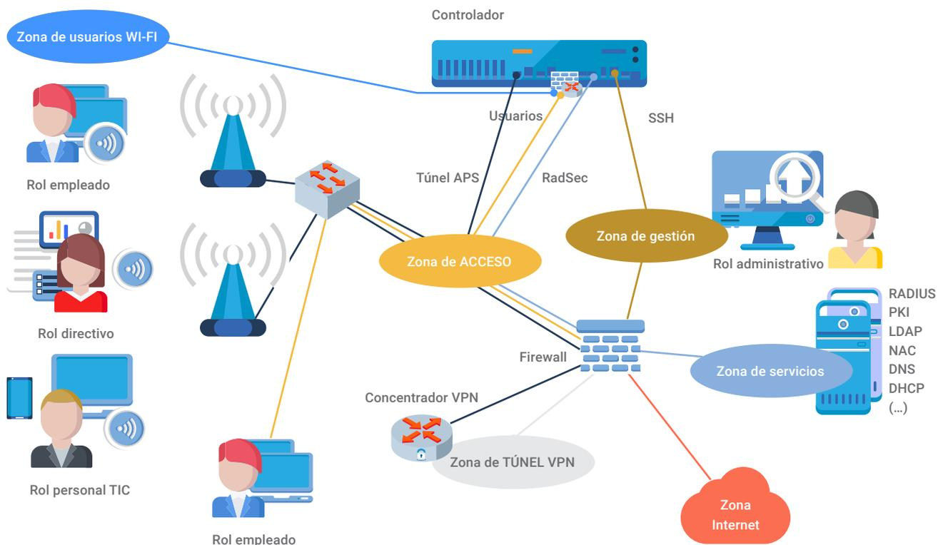
If it is decided that the controller will act as a level 3 equipment (performing routing tasks) two zones can be defined in the controller for the users: Wi-Fi user network zone and corporate access network zone.
