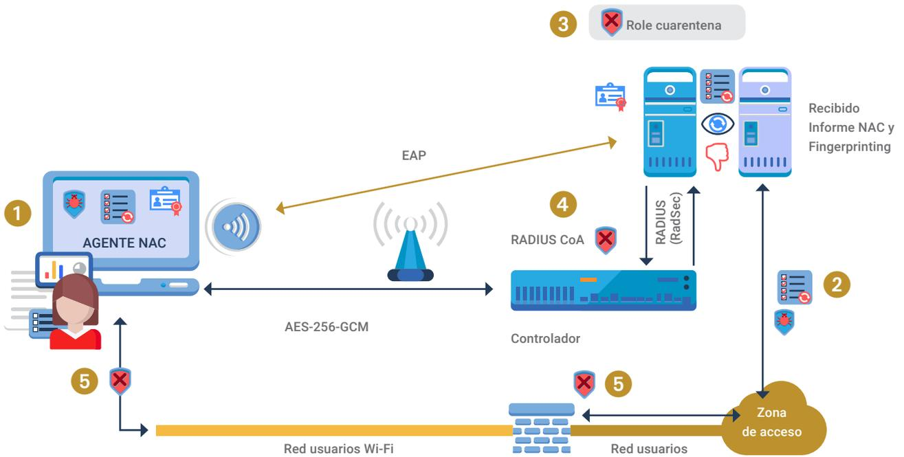
If, on the other hand, the report indicates that it does not comply with the security requirements, it will switch to "**quarantine role**", restricting access to the minimum services required to solve the problems detected (**Figure 10**).
